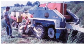
Machine built by Dick Harris uses deep ripper shanks that mount in front of planter row units. Big tires tamp down the soil to keep the surface smooth.
