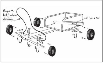
Wooden push cart rides on rubber tires with inset bearings that fit a 5/8-in. steel shaft.
