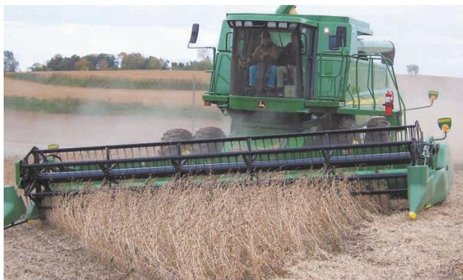
New sidehill leveling kit, designed for Deere STS combines, allows the leveling system to operate with minimal change to the machine.
