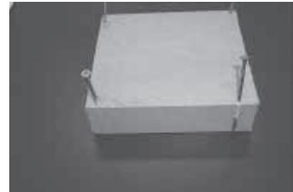
Boards can be nailed, glued, stapled or screwed without splitting.
