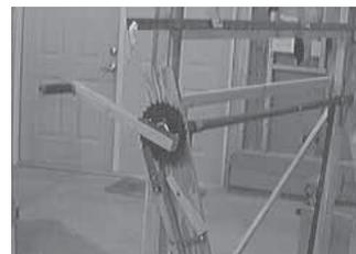
Ratcheting mechanism consists of an old circular saw blade and an angle iron "ratchet" with a spring attached to it.
