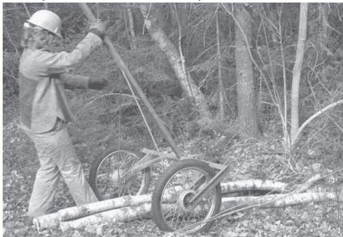
Tipping the sulky back lowers the frame to the log, which is then chained in place. Photos courtesy University of Maine
