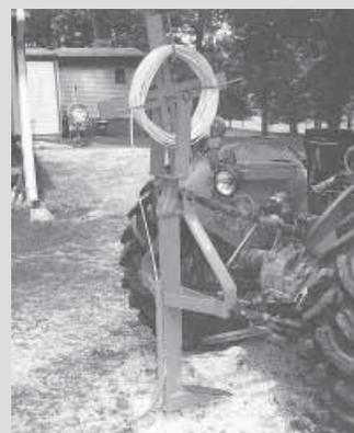
Feilbach bent a piece of 1-in. pipe 90 degrees and then welded it to the back of the subsoiler, with the end almost as far down as the blade.
