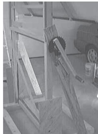
Wood frame that holds drywall mounts on two wooden uprights that slide up or down inside wooden guides.
