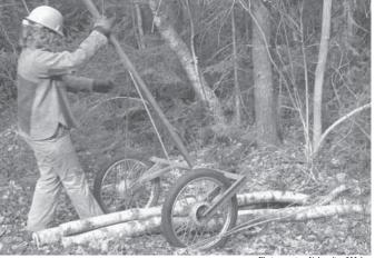
Tipping the sulky back lowers the frame to the log, which is then chained in place.
