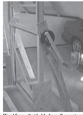
Wood frame that holds drywall mounts on two wooden uprights that slide up or down inside wooden guides.
