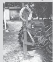
Feilbach bent a piece of 1-in. pipe 90 degrees and then welded it to the back of the subsoiler, with the end almost as far down
