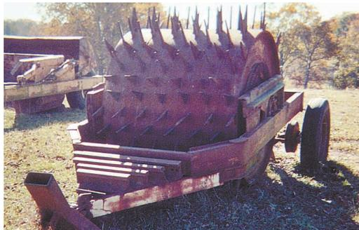
Massive aerator has a drum 5 ft. long and 5 ft. in diameter that's made of 1-in. thick steel.
