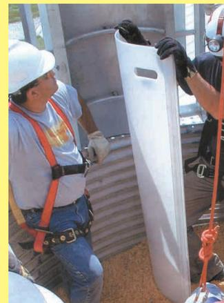
Rescue workers fit the tube together inside the bin, then drive the panels down into the grain.
