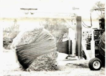
When bale is wrapped, machine automatically cuts off plastic and tucks in loose end.
