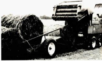
Driver can discharge 3 bales at any point in field by pulling a rope before 4th bale is formed.
