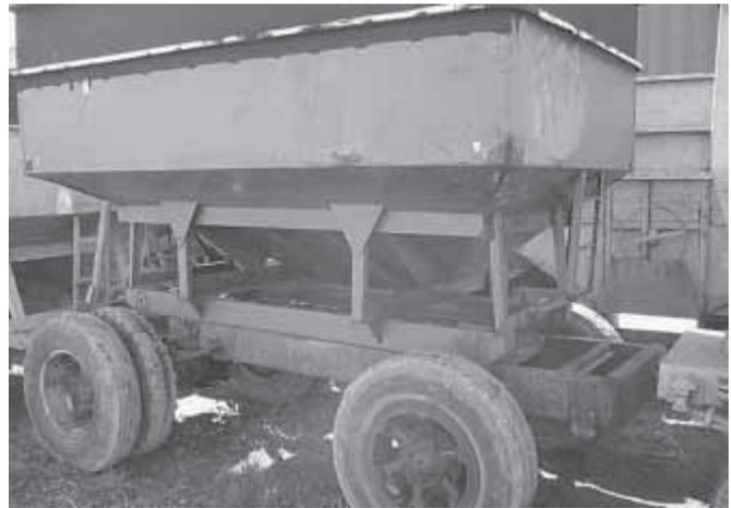
This 225 bu. wagon was built using axles off a 2-ton International truck.
