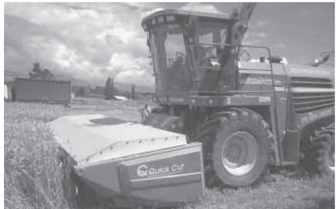
With mower header, Bruce travels 12 to 15 mph in a light crop and still makes a nice, clean cut.
