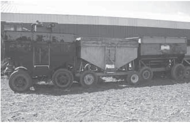
Wagon shown at left was built using the axles off a Ford F-600 2-ton truck. Middle wagon was built from scratch using two Massey combine axles. Front axle on wagon at far right is off an F-600 Ford 2-ton truck; the rear axle is a concrete mixer's tag axle.
