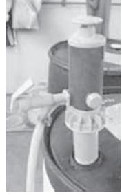
Hand pump pressurizes a container with a few strokes of the piston. Then you tap down on a "faucet" to dispense liquid in precise amounts, adjustable up to 4 1/2 gal. per minute.
