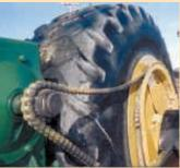
Plate on side of tire hinges open to add and remove rocks.
