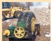
A 3 hp, 220-volt electric motor with a variable speed pulley drives a gearbox, which chain-drives a 28-in. sprocket mounted on one side of tumbler.
