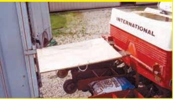
To make it easier to fill my IH air planter, I mounted a pipe bracket across the back of the hopper. When I back a grain trucked filled with seed pallets up to the planter, I slide two 2 by 6's with hooks on them out of the truck to hook over the
