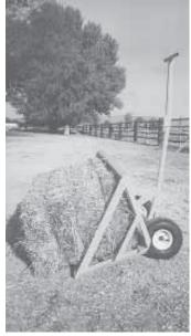
After lifting bale, cradle turns 90 degrees so you can push cart through narrow doorways or gates.
