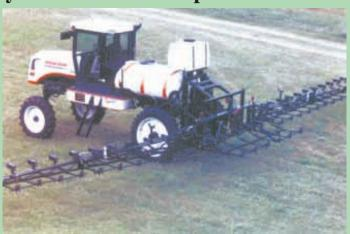
GreenSeeker system "reads" the nitrogen needs of crops on-the-go and only applies what is needed. It's shown here with optical sensors and variable rate nozzles mounted on a 60-ft., self-propelled sprayer.
