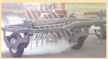
Machine creates "artificial dew" by injecting water with a softening agent added. Tines on reel poke down into windrow and spray in a fine mist.
