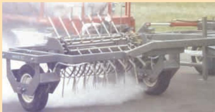
Machine creates “artificial dew” by injecting water with a softening agent added. Tines on reel poke down into windrow and spray in a fine mist.
