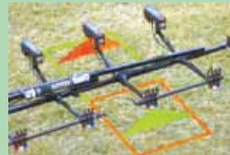
Sensors measure nitrogen needs in a 2-ft. sq. area. A microprocessor circuit board analyzes the reflected light and determines whether to activate the spray nozzles for that 2-ft. sq. area and, if so, how much material to apply.
