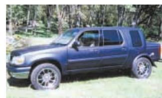
Vehicle's trunk was fabricated from the bed off a 1988 Ford pickup. The tonneau cover on top was fashioned from the hood off a 2001 Explorer.
