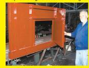
one didn't let the grain flow out fast enough. The new door lets grain flow 1 1/2 times faster. I also put the door latch low so anyone can open it. If I wanted to, I could cut a slide in it to insert an auger (Clair Wilson, Winchester, III.)
