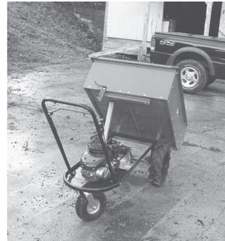
Home-built wheelbarrow is powered by a 6 1/2 hp garden tractor engine and hydrostatic drive unit. The 48 by 30 by 15-in. deep box is balanced for easy dumping.
