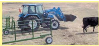
To catch a cow with tractor-pulled "cow catcher", driver extends a cylinder to swing one side of corral out about 30 ft. away from tractor.
