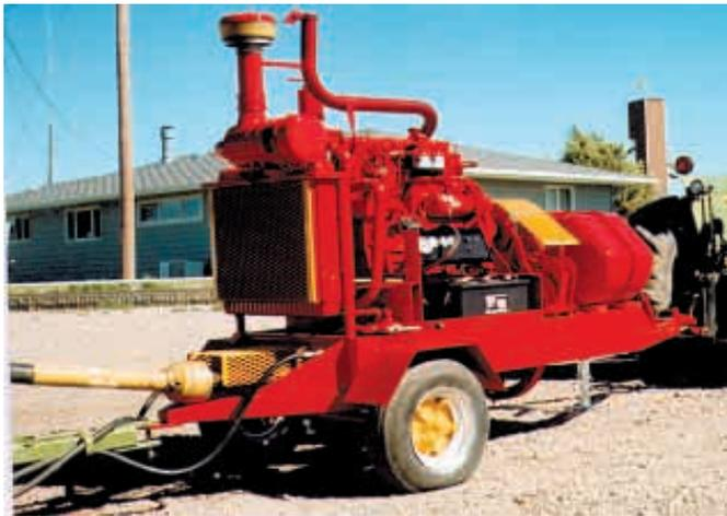
Portable pto works for anyone without a tractor or who has more pto work than they can handle. Benjamin used a diesel, but a smaller model could use an electric motor.
