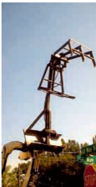
Grapple grabs debris and lifts it high to reach over truck boxes.
