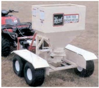
High-flotation broadcast spreader is equipped with four flotation tires which keep spreader from doglegging on hillsides.
