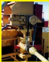
Belt runs from a specially machined pulley on gearbox to main shaft on mill. "The machine runs real quiet," Weaver says.
