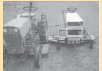
Davis pulls the wing mower alongside his Power King garden tractor, which has a 4-ft. deck. Four caster wheels allow the wing mower to move in any direction with the Power King.
