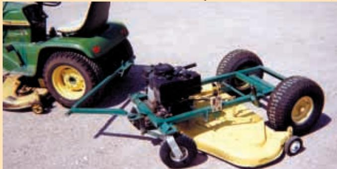
Richard Moore mounted the deck off a junked Deere 112 riding mower on a wheeled frame. He uses a Tecumseh 10 hp engine to power the trailing deck.
