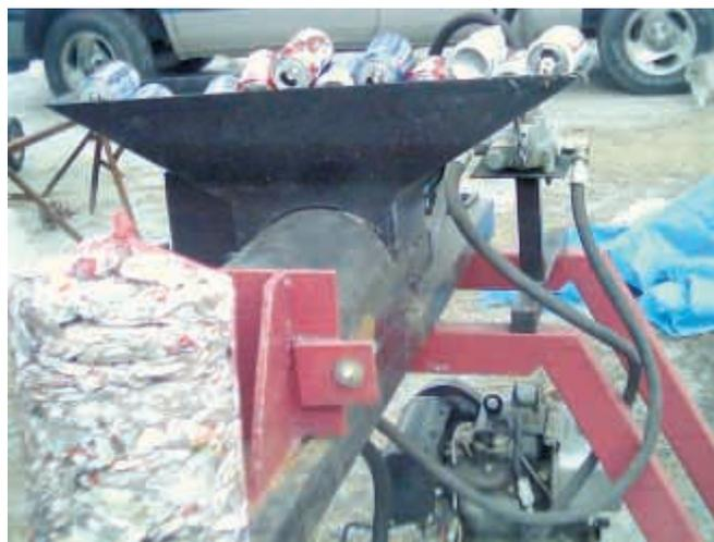
Log splitter attachment has a hopper that allows it to crush a bunch of cans at once, rather than one at a time like most crushers.
