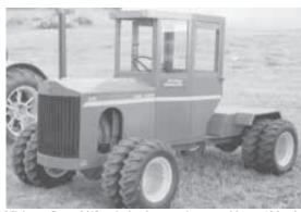
Miniature Deere 2418 articulated tractor is powered by an 18 hp, 2-cyl. LUC gas engine off an old Deere A12 combine.
