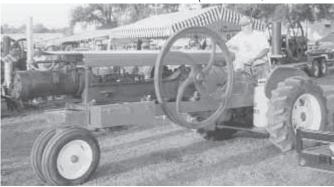
Hunter mounted a Thomas "half-breed" oil field engine on a stretched-out 1936 Allis WC tractor. Note big 4-ft. dia. flywheel on one side and water cylinder on front.
