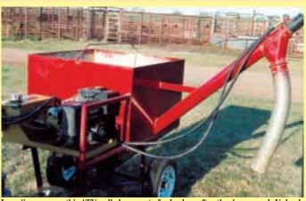
Leon So wers uses this ATV-pulled wagon to feed calves after they're weaned. Unloading auger is powered by hydraulic power unit that's driven by an 8 hp gas engine.
