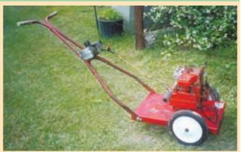
Engine mounts on the frame of an old pressure washer. Insecticide is stored in a small plastic tank mounted on rig's handles.
