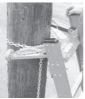
V-shaped safety device clamps to top rung of extension ladders. Spike bars grip trees and poles. Apair of hinged, round pads at either end keep ladder from sliding on flat surfaces.
