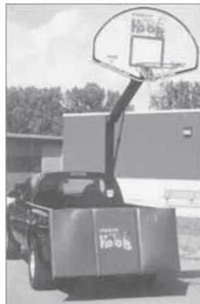
Pickup-mounted hoop folds down for transport. It's adjustable from 6 to 10 ft. high.
