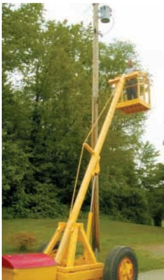
Bucket attaches to end of 19-ft. long boom, which is made of 6-in. dia. steel gas pipe.
