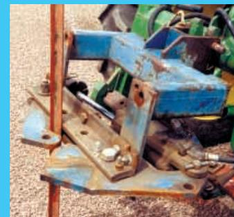
Post puller consists of a steel jaw that's hinged in middle and is attached to a hydraulic cylinder. Extending the cylinder closes jaw around post.
