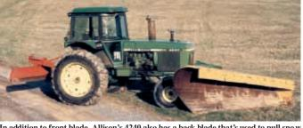
In addition to front blade, Allison's 4240 also has a back blade that's used to pull snow away from buildings.
