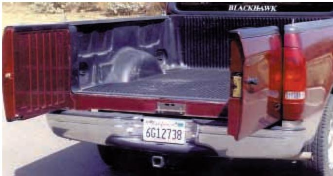
Two-piece "double door" tailgate opens from both sides, making it easy to load items onto bed.
