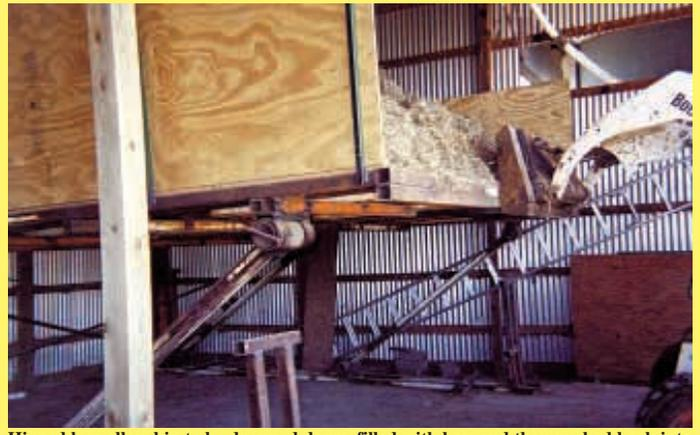
Hinged legs allow bin to be dropped down, filled with hay, and then pushed back into upright position with a skidsteer.
