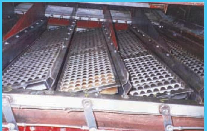
Sieve replaces combine's original chaffer sieve and is fitted with rigid steel deflectors that separate chaffer sections.
