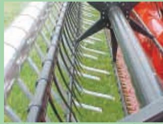
Out-front manifold puts nozzles down between reel fingers, ahead of knife.
