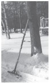
Lothe's 76-in. long "tree jack" consists of a heavy duty screw jack attached to pieces of sq. tubing. He extends the jack to push
