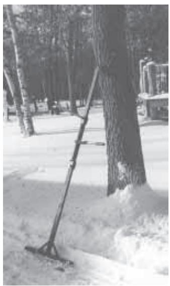
**Lothe's 76-in. long "tree jack" consists of a heavy duty screw jack attached to pieces of sq. tubing. He extends the jack to push tree over.**
