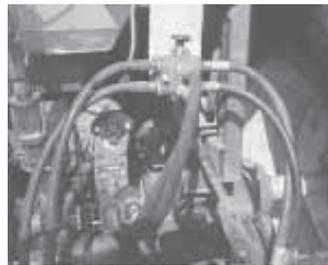
from Northern Tool Equipment (ph 800 556-7885) allows us to use one remote outlet on our tractors to operate two hydraulic cylinders. The valve costs less than \$100, compared to electric/hydraulic converters that that can cost up to \$500.
