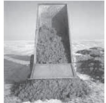
Box is raised and lowered by a pair of 5-in. dia. hydraulic cylinders. A scissors-action lever at back of box is used to release tailgate.
