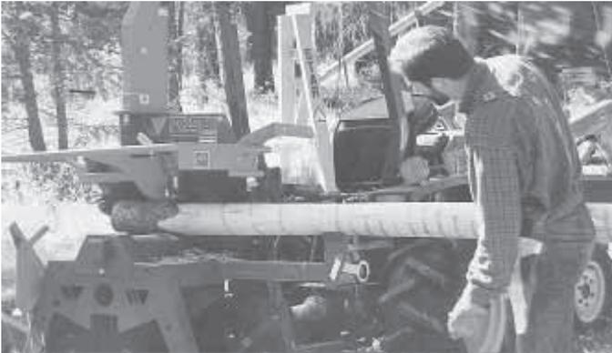
Post peeler automatically pulls log past a 22-in. dia. disk equipped with four 6-in. knives. They take off bark, leaving post smooth and round.
