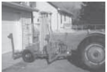
Two-wheeled rig is equipped with a stand-in cage and four outriggers.
