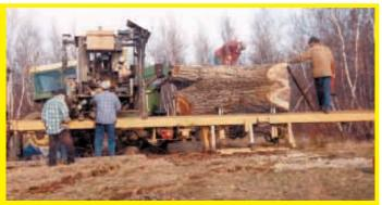
My home-built sawmillwill handle the biggest, toughest logs. It's powered by a 50 hp. Cummins Onan engine, which runs the bandsaw blades and debarker. An 11 hp. Honda engine runs all hydraulics on the log carriage itself. The saw's operated by 32 switches.Our best 2-day run with the sawmill was 12,128
