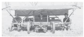
Aspargus machine was made from the wide front axle off an Allis Chalmers G tractor and the rear end of a pickup.
