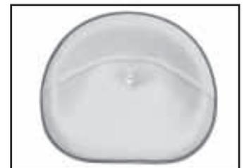
Farmall pan seat cushion has a steel core and a brass drain hole.
