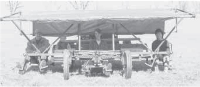
Asparagus machine was made from the wide front axle off an Allis Chalmers G tractor and the rear end of a pickup.
