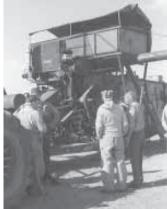
Machine's hopper and unloading auger is off an old Case pull-type combine. The hopper was enlarged by cutting the sidewalls away from three hoppers and then welding them together.
