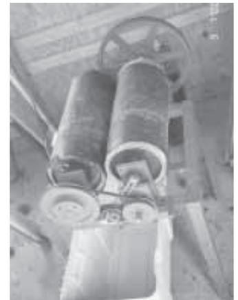
Home-built chestnut dehusker consists of two 3-ft. long, 8-in. dia. padded drums that rotate at slightly different speeds, providing the friction to rub off prickly husks.
