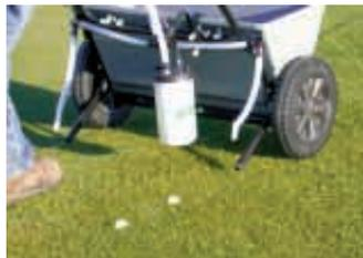
Marker has a single 32-oz. tank and a small air pump powered by a D-cell battery.
