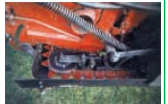
Photo of Loftus's original sicklebar shows continuous cutter chain equipped with replaceable sickle sections.
