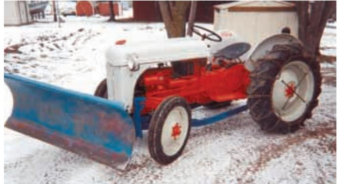
Seven-foot blade is supported by steel subframe that attaches under tractor and extends all the way to the hydraulic lift on back.
