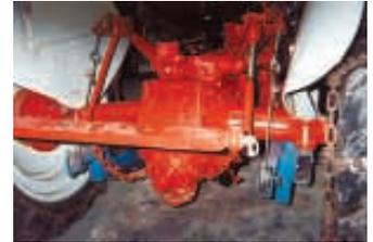
Cables are connected to upper part of tractor's hydraulic lift arms.
