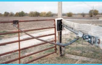
Kent Elder uses ordinary garage door openers to build his automatic gate openers. "The toughest part is finding the right angle for the opener rail support," he says.
