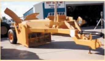
Triple "S" Ditcher cuts a 60-in. wide flat-bottomed drainage ditch that's up to 6 in. deep.
