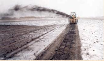
Blower spreads soil without leaving a berm on either side of ditcher.
