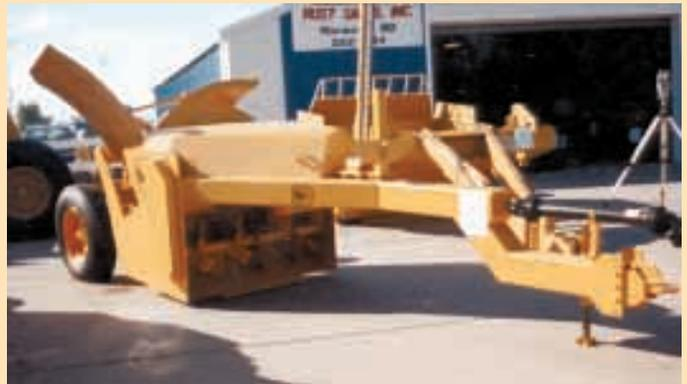
Triple "S" Ditcher cuts a 60-in. wide flat-bottomed drainage ditch that's up to 6 in. deep.
