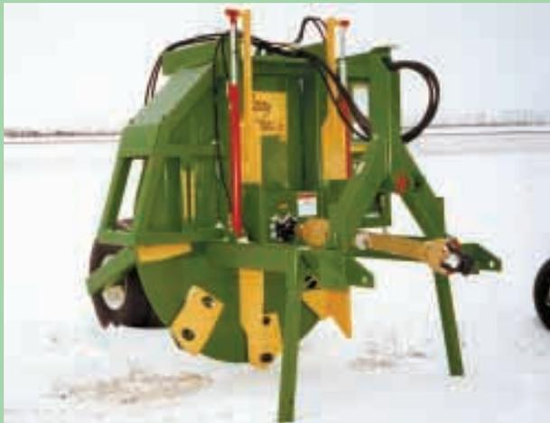
Heavy-duty ditcher can be equipped with either a 42 or 72-in. dia. flywheel.
