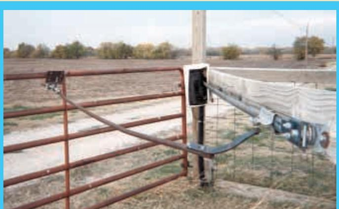
Kent Elder uses ordinary garage door openers to build his automatic gate openers. "The toughest part is finding the right angle for the opener rail support," he says.
