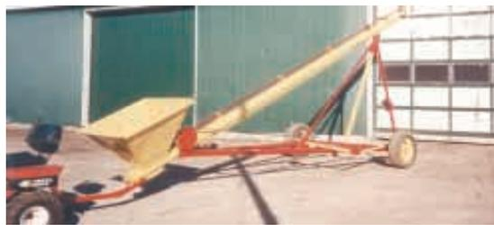
Van Soest's 22-ft. "drill fill" auger has a big steel hopper and a short tongue welded onto the bottom end, allowing him to use a garden tractor to move it around.
