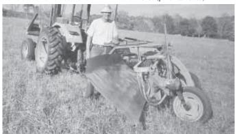
A 3-ft. wide tray mounts on front of Gannon's New Holland 256 basket rake, about 6 in. off the ground. When rake teeth pick up windrow to roll it, the tray catches it and slides the hay off the back onto drier ground.
