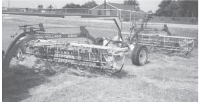
**Nutting doubled up two New Holland 9-ft. side delivery rakes. An 18-ft. long "bridge hitch" connects the two rakes.**
