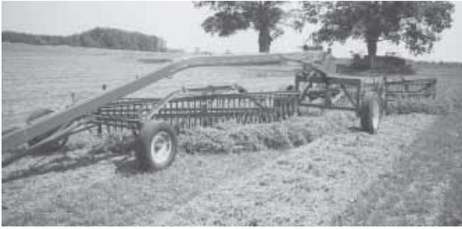
**Tandem rake hitch was made from two Deere side delivery rakes and the tongue from a hydroswing haybine.**
