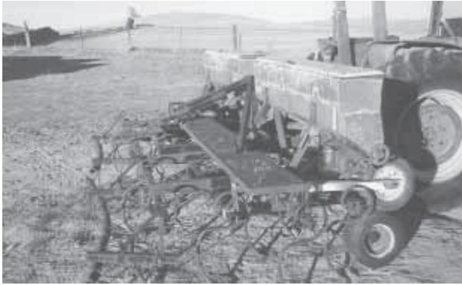
Mounting a pair of dry fertilizer applicators onto his 3-pt. mounted field cultivator lets Edwin Egli do all his tillage, seeding, and fertilizer work in one pass (drill not shown).
