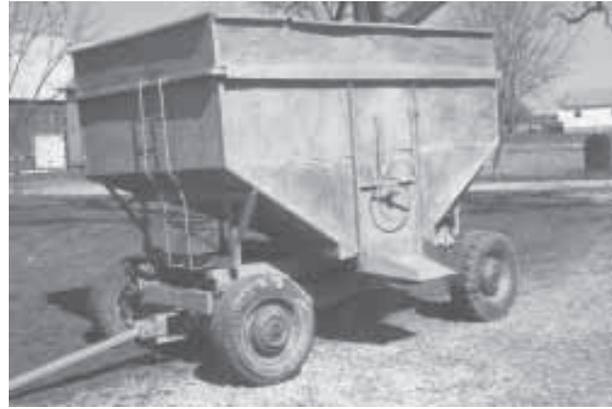
Stadler started with the frame of a 1978 Ford F-350 pickup and mounted a 175-bu. Killbros gravity wagon on it.
