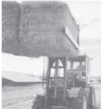
Tractor's Freeman squeeze mast is shown here with two 4 by 4 by 8-ft. bales, but it can actually handle four bales at once.
